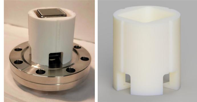
Has been printed in PLA and PETG, will eventually be printed in **resin** (radio pure material)
